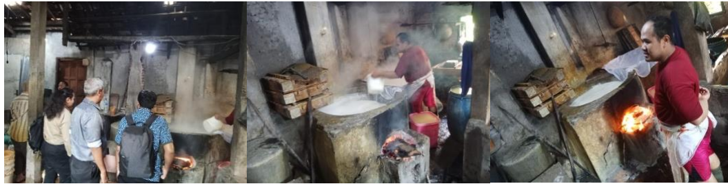
Figure 1. Initial combustion system and production layout at UD SDD Kediri.
