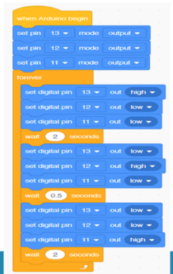
Fig. 1 C Programming, block to turn on the LED
